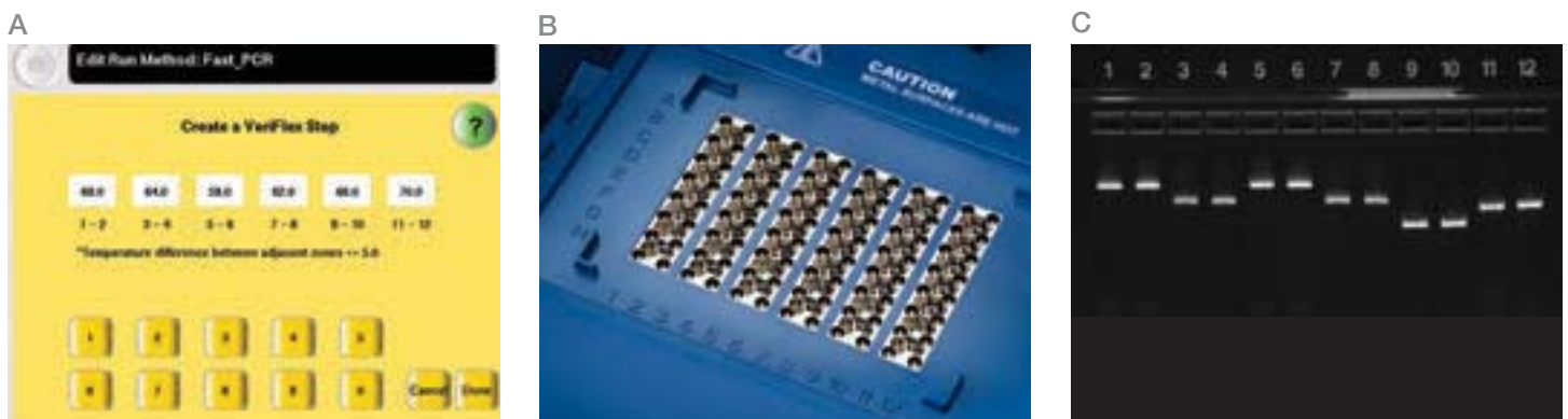
Figure 1. Applied Biosystems thermal cycler technology. (A) Applied Biosystems™ Veriti™ 96-Well Thermal Cycler software shows annealing temperatures set for six different primers. (B) VeriFlex Blocks: six individual Peltier blocks. (C) PCR results showing six primer sets run in a single PCR amplification cycle. The Veriti 96-Well Thermal Cycler can run six assays at six annealing temperatures during the same PCR run.
